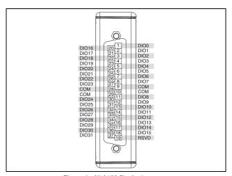
Figure 1. NI 9403 Pin Assignments
